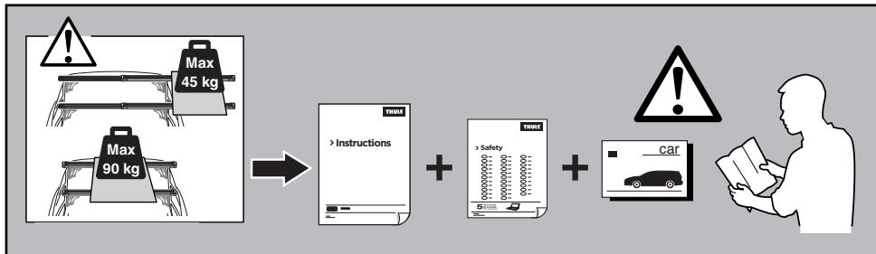
**GB** Maximum load Thule SlideBar = 90kg, or less if stated differently in roof rack- or car instruction manual.
